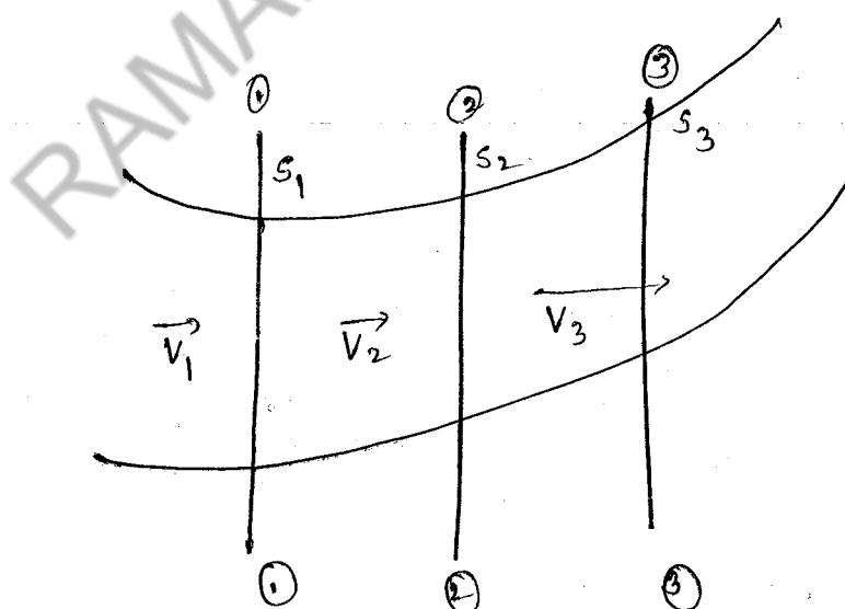
$S_1, S_2, S_3$  are cross sectional area,  $V_1, V_2$  &  $V_3$  are velocities at ①-① channel, ②-② channel & ③-③ channel
